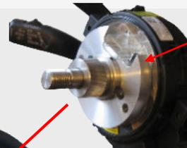
Measuring steering wheel on shaft put on and screw together; Cover put on.
