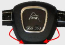
Z5/Z7: open the hook-and-loop tape and draw off cover forwards.
