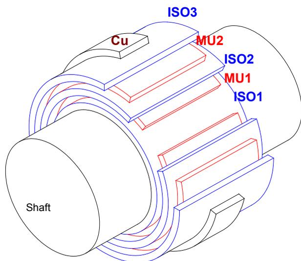
The final insulation will depend on the environment. Any covering or waterproofing should be non-conductive. For extended temperature range the covering should be Kapton high temperature tape (supplied) and if there are very high acceleration loads a covering with epoxy-glass cloth is recommended.
