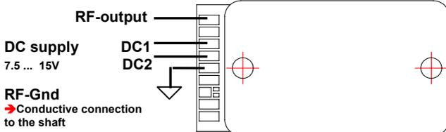
**Polarity of DC supply is random, because a rectification is integrated**
