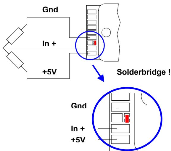
Using the **K1-M2** electronics the thermo couple is to connect to the pads In+ and In-.
